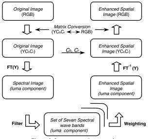
Figure 1. Image processing operations
